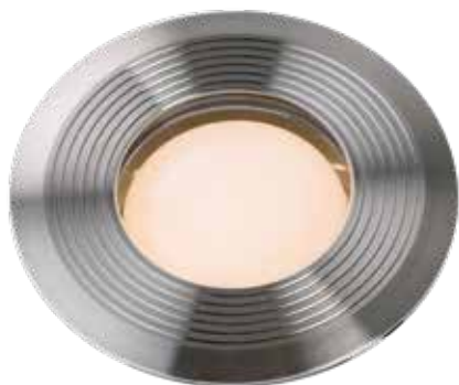
Onyx 90 R1 [156D] Stainless steel 316 LED 1,5W 2.700K - 76lm 43 x 105 mm (HxØ) Drillhole: 90mm
