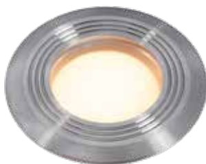
Onyx 60 R1 [151D] Stainless steel 316 LED 1W 2.700K - 23lm 42 x 75 mm (HxØ) Drillhole: 60mm
