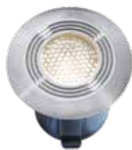
Onyx 30 R1 [150D] Stainless steel 316 LED 0,5W 2.700K- 4lm 41 x 45 mm (HxØ) Drillhole: 30mm
